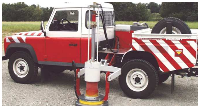
Figure 4 : Dynaplaque (photo : Vectra)
