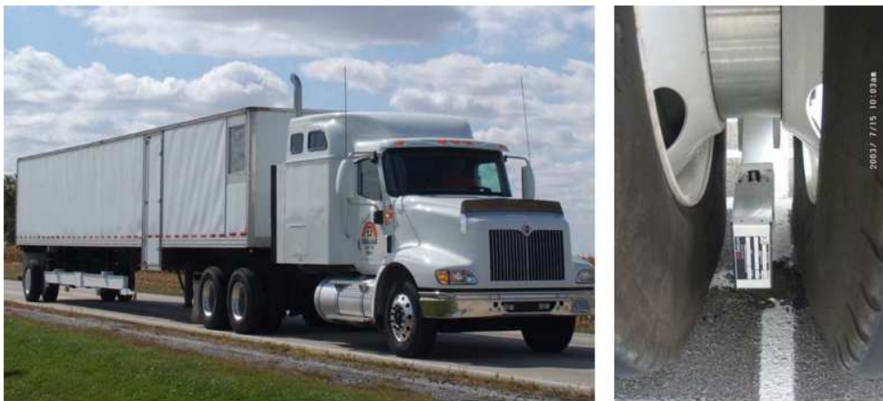
Figure 8 : Rolling Wheel Deflectometer (photo : [STEE08])
