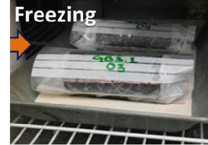
Specimen in a plastic bag with 10cl water
